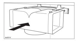
Slide the diverter on to the brackets of plate B.
